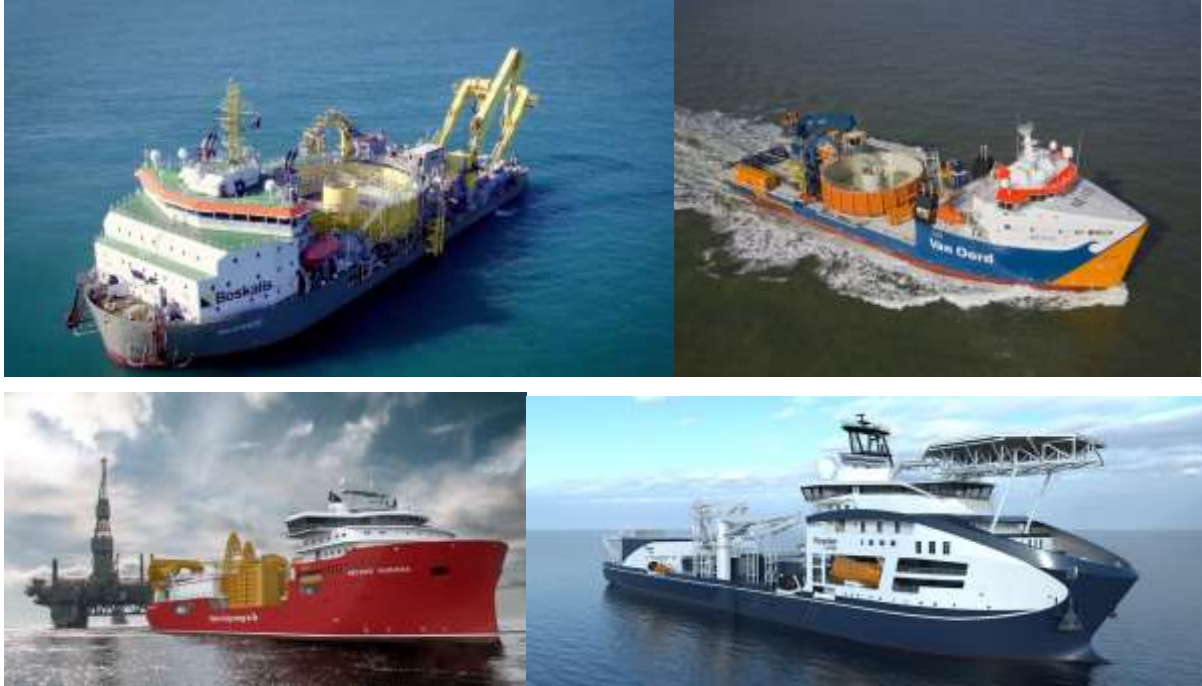
Figure 2.30 Typical Cable Lay Vessels
