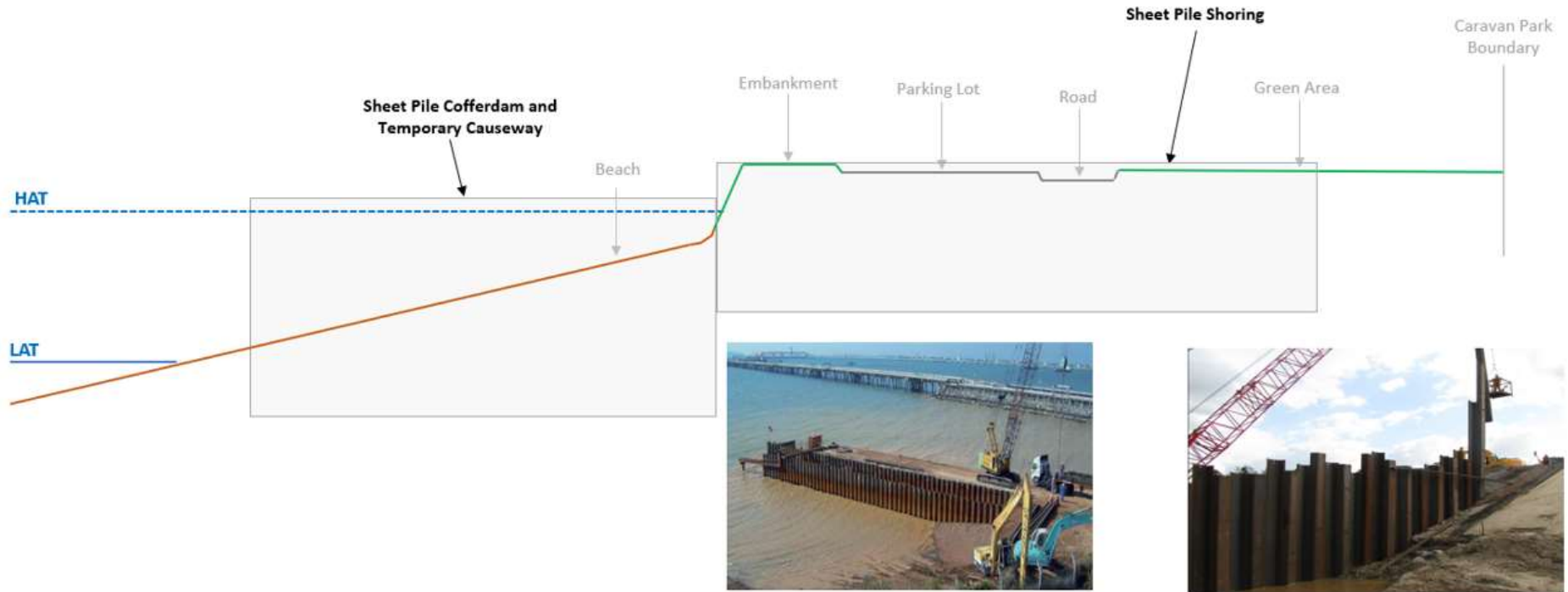
Figure 2.6 Temporary Works – Cofferdam and Causeway Construction
